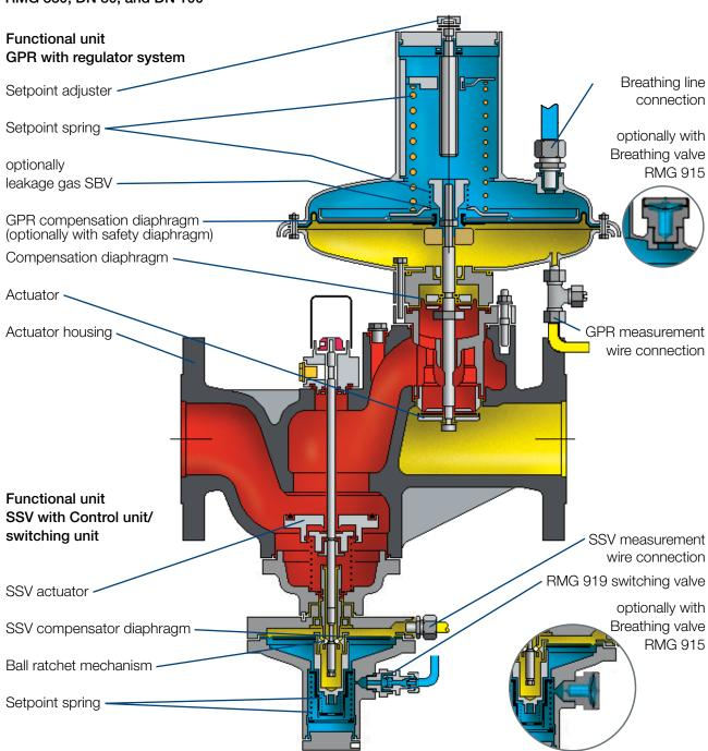
The compensation diaphragm of the regulator records the actual value of the outlet pressure and compares it with the set value specified by the setpoint spring. A regulation deviation has a direct influence through the valve rod to the actuator position. The resulting change in flow causes an equalization of the actual outlet pressure value with the setpoint. At zero consumption, the device seals tight and the closing pressure is set.
